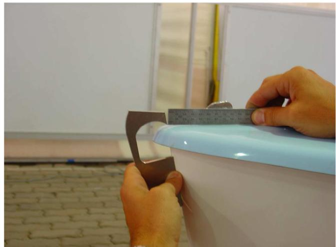
(from the transom to the FMP) and the jib wire hole position is measured backwards with a ruler. The value should be the same as the one in the measurement form.
