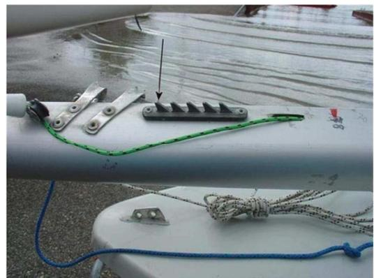
Solution No3: Screw, rivet or other obstacle inside the sail track. This is an easy solution for masts with rope halyards and a clam-cleat.
