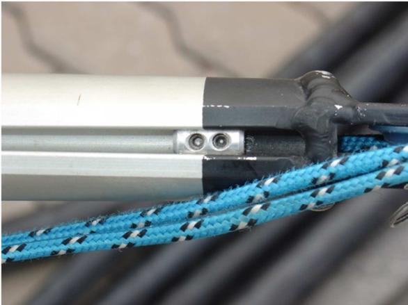
A rivet, screw etc inside the sail track is also a common and easily made stopper for the boom outer limit point as well, as shown in the following picture:
