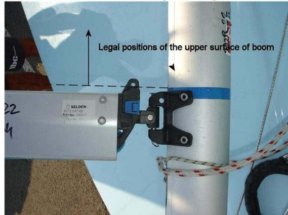
The upper boom surface cannot be set below the “lower point”, which is the top point of the limit mark on the aft mast edge. Possible solutions for this kind of problem include:
