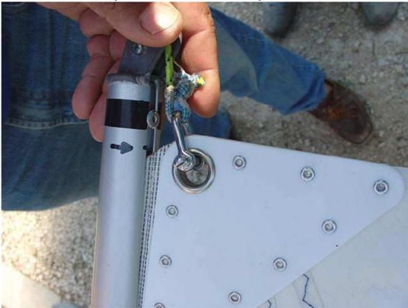
A RIVET USED AS A STOPPER CAN EASILY DAMAGE THE MAINSAIL, CUTTING THROUGH THE TABLING AND NEGATING THE STOPPER EFFECT AFTER A FEW DAYS OF RACING. SOLUTIONS LIKE THE ONE SHOWN BELOW ARE MUCH BETTER.
