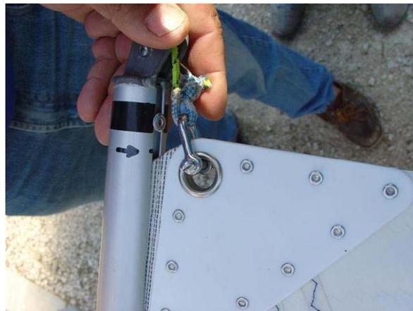
ADVICE! A RIVET USED AS A STOPPER CAN EASILY DAMAGE THE MAINSAIL, CUTTING THROUGH THE TABLING AND NEGATING THE STOPPER EFFECT AFTER A FEW DAYS OF RACING. SOLUTIONS LIKE THE ONE SHOWN BELOW ARE MUCH BETTER.
