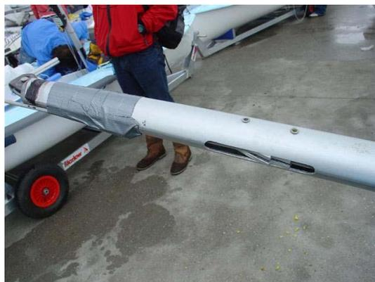
Solution No2: Tooth rack (for wire halyards only). If you use the last position (as shown by the arrow) or if there is only one, then it acts like a stopper, since you have only one possible position for the mainsail like the masthead lock. If the correct position for the halyard is the middle one for example, you must cut out the remaining teeth, or use another stopper solution.
