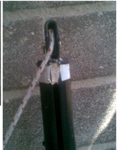
In these examples, the stoppers are positioned for mainsails with square-cut boltrope at the head. In the following picture, you see that if you change into a mainsail with cut-down boltrope, then the stopper for a normal mainsail will not work because the mainsail can be set higher than the limit point. In that case the stopper must be installed in the position shown by the arrow in the following picture:
