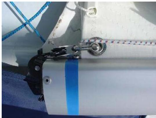
In this example of a boom stopper, the rivet has been installed a few mm inside the limit. Again, the exact position of the stopper depends on the shape of your sail's clew. Sometimes there is a slider which extends outwards: in that case, the stopper may be positioned outside the limit mark because any attachment like a slider is ignored for measurement purposes. Again, check your particular mainsail first and then position the stopper!
