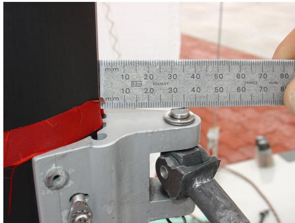
3. Spinnaker halyard cranes are to be positioned so that no part of the fitting itself is more than 60 mm from the mast spar. The measurement is taken to the outmost point of the fitting as a whole and not to the bearing point of the rope halyard!
